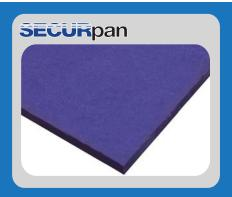
SECURpan is a unique fiberboard roofing insulation panel whose core has been thoroughly treated to provide fire-resistance. SECURpan is a certified UL 790 Class A and FM approved Class 1 material.
